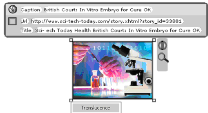
Figure 4: In-context metadata details on demand above an image surrogate. We see fields for the image (top row) and for its container (rows 2, 3). In this case, there is no hyperlink. In-context tools to the right afford latching and search. The edit palette, below, enables editing of visual attributes, such as translucence in the case of image surrogates.
