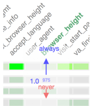
Figure 5: Seeing the value 975 on the browser field, the user clicks, then drags up to add browser = 975 as a term to the query.
